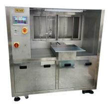
The client wanted to add automation functionality to their existing spray machine. We designed a dual-axis servo platform to allow programmable spray range control. The system supports adjustable movement speeds, one-way or two-way spraying, and both intermittent and continuous spray modes.
