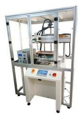
The client required bulk plasma treatment for SD cards. We designed a plasma machine with an XY servo platform, a lifting module, and a blower system to prevent parts from being displaced during treatment.
