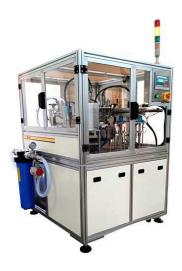
Cleaning is critical in the contact lens manufacturing process. We provided a precision 6-station rotary indexing table with inverter-controlled positioning and pump/filtration systems to ensure clean water quality.
